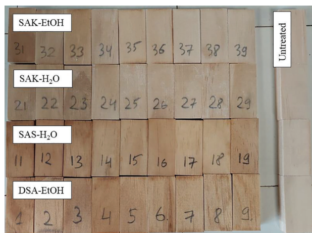
Figure 8: Visual appearance of the impregnated samples after leaching and drying
