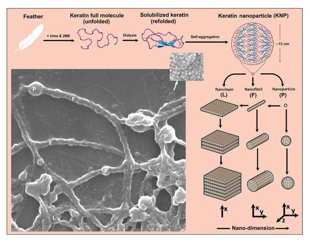
**Figure 5:** A schematic diagram demonstrating how keratin nanoparticles can be formed and served as the building blocks for higher nanostructures. Letters P, F and L indicate nanoparticles, nanofibrils and nanolayers, respectively (Reproduced with permission from Reference [133], © Elsevier 2020)
