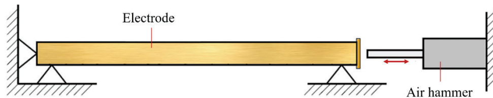
Figure 6: An electrode-forming apparatus that detects the electric field across surfaces. Adapted with permission from Reference [70], Copyright © 1963, Forest Products Society
