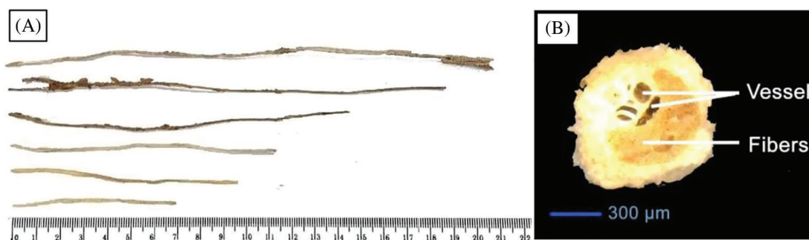
Figure 1: Oil palm trunk vascular bundles, (A) longitudinal section and (B) cross-section
