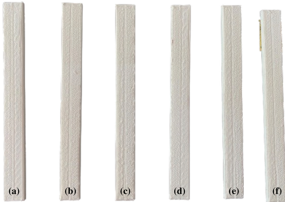
Figure 6: Flexural test samples with: (a) 0, (b) 10, (c) 20, (d) 30, (e) 40 and (f) 50% reinforcements
