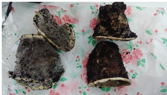
Figure 1: Degradation of paper of the paper cups using Eisenia fetida . Cups to the left were subject to Eisenia fetida degradation. Cups to the right were not subjected to Eisenia fetida degradation
