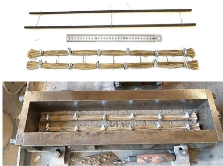
Figure 10: Hybrid concrete beams made from steel and OPBF strands. Adapted with permission from Reference [77]. Copyright © 2024, Elsevier Ltd.
