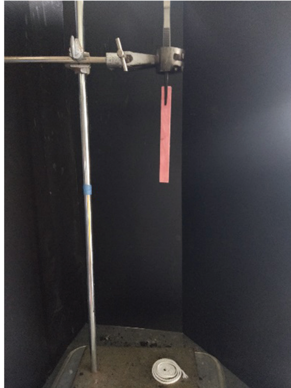
Figure 4: Experimental set up for the UL 94 VB test
