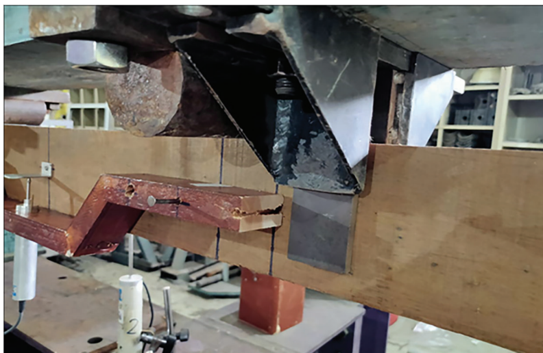
Figure 2: Setup for bending test with bracings for specimens with the length of 2000 and 2500 mm
