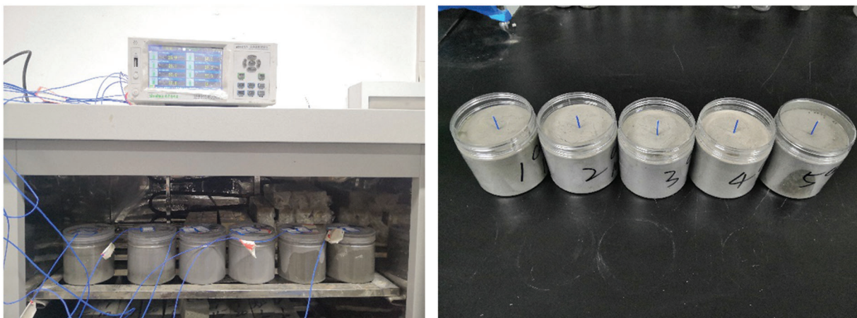
Figure 2: Hydration temperature testing device and test samples
