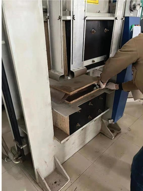
**Figure 3:** Cold pressing process of composite plywood
