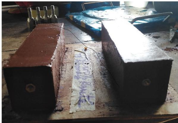
**Figure 6:**  $4 \times 4 \times 16$  specimens with inserted studs
