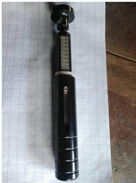
**Figure 4:** Pocket penetrometer
