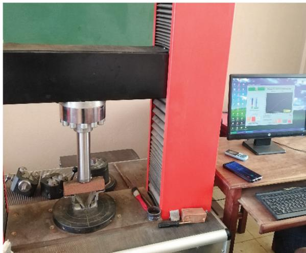
**Figure 8:** 3 points bending tests
