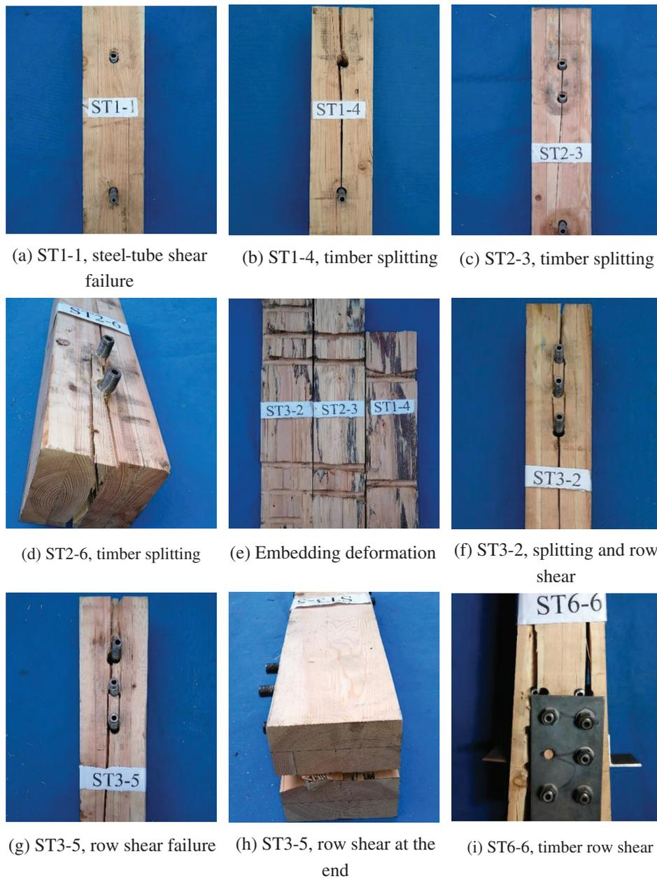
**Figure 7:** Failure photographs of STS specimens with large diameter steel-tubes
