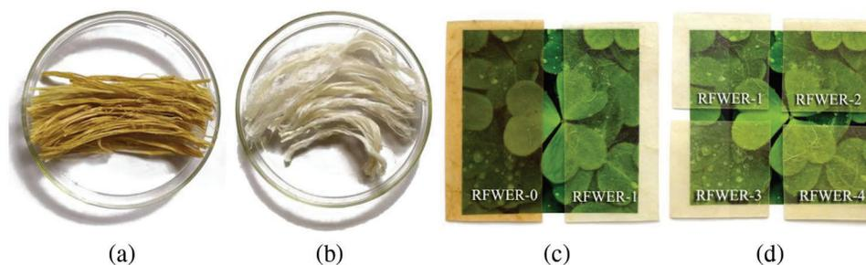
**Figure 2:** Untreated ER (a) and NaClO<sub>2</sub>-treated ER (b). Untreated and NaClO<sub>2</sub>-treated composites (c) and Composites with different number of pressed layers (d)
