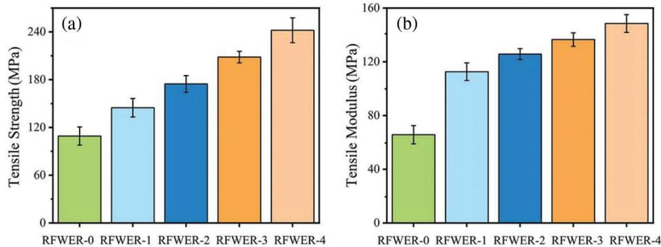
**Figure 4:** RF/WER composite tensile strength (a) and tensile modulus (b)
