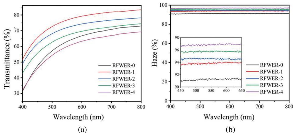
**Figure 3:** RF/WER composite transmittance (a) and haze (b)
