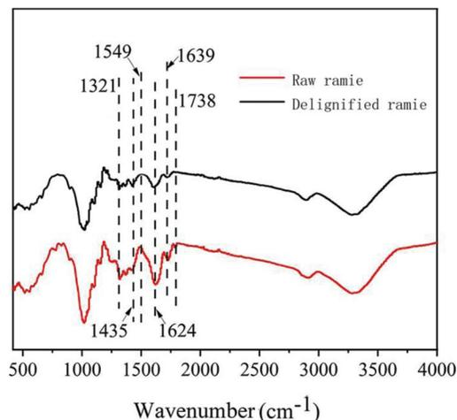
**Figure 6:** Infrared spectra of RF before and after  $\text{NaClO}_2$  treatment
