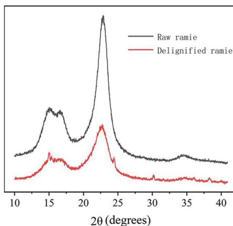
**Figure 7:** XRD patterns of RF before and after  $\text{NaClO}_2$  treatment
