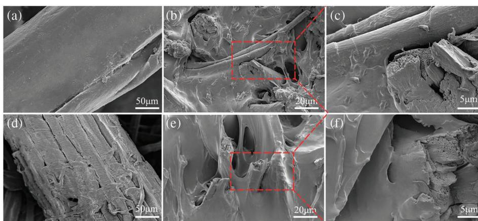
**Figure 8:** SEM images of untreated RF (a) and NaClO<sub>2</sub>-treated RF (d). SEM images of untreated composites (b), (c) and NaClO<sub>2</sub>-treated composites (e), (f)
