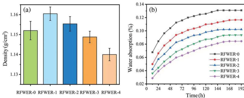
**Figure 5:** RF/WER composite density (a) and water absorption (b)
