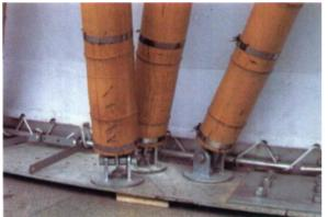
**Figure 21:** Connection between raw bamboo and floor [34]
