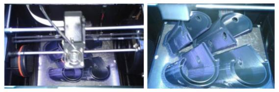
Figure 34: 3D printing 1:1 scale joints [72]
