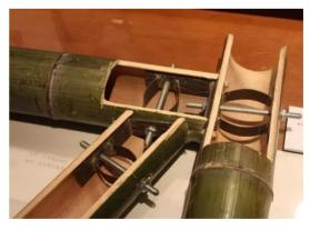
Figure 10: Wang Shu jointing method [34]
