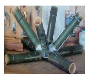
Figure 16: Steel plate joint [28]
