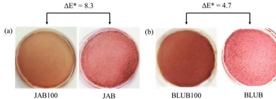
**Figure 3:** Visual aspect and total color difference values between the corn starch based films: (a) JAB100 and JAB ( $\Delta E^* = 8.3$ ) and (b) BLUB100 and BLUB ( $\Delta E^* = 4.7$ )
