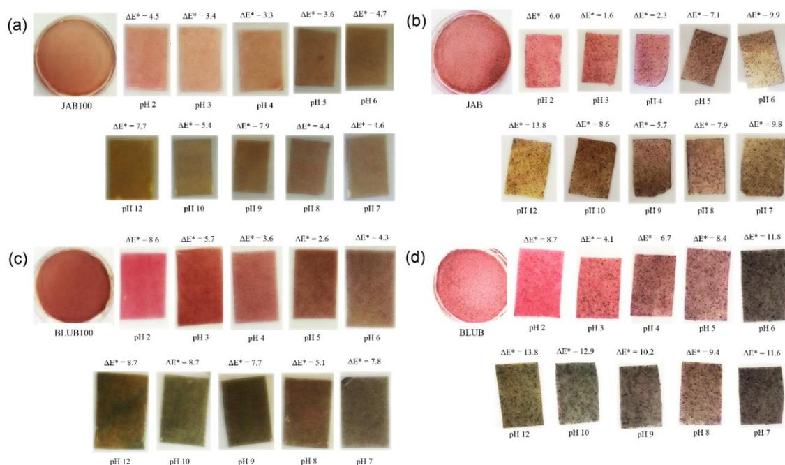
**Figure 4:** Visual aspect and total color difference after immersion in different pH values between the corn starch based films: (a) JAB100 (jaboticaba residue fraction that passed through the sieve of 100 mesh), (b) JAB (jaboticaba residue fraction retained in the sieve of 100 mesh), (c) BLUB100 (blueberry residue fraction that passed through the sieve of 100 mesh), and (d) BLUB (blueberry residue fraction retained in the sieve of 100 mesh)
