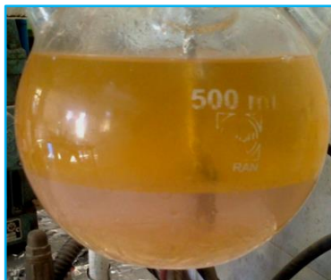
Figure 1: The phase separation in bilayers after adding silica gel at the end of the epoxidation process
