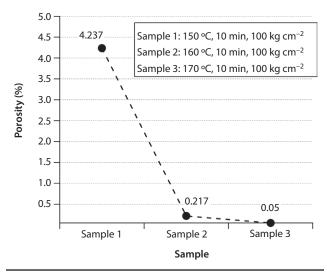
Figure 3 Porosity in banana fiber-reinforced composites processed at various temperatures.
