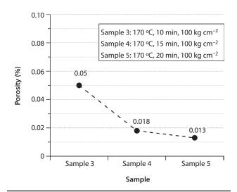
Figure 6 Porosity in banana fiber-reinforced composites processed in various times.
