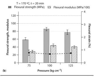
**Figure 8** Effects of processing pressure on (**a**) tensile and (**b**) flexural properties of banana fiber-reinforced composites.
