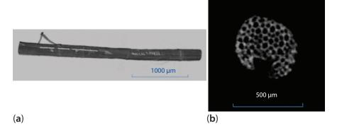
Figure 1 Structure of banana fibers observed by X-ray CT (a) along the length and (b) at cross section of the fibers.
