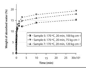
Figure 11 Water absorption of banana fiber-reinforced composites processed under various pressures.
