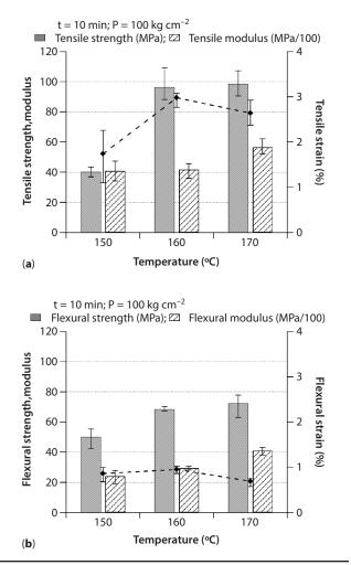
**Figure 2** Effects of processing temperature on (**a**) tensile and (**b**) flexural properties of banana fiber-reinforced composites.
