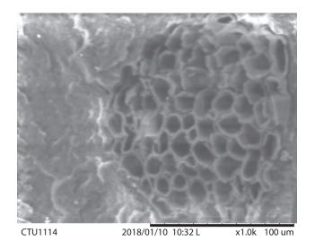
**Figure 13** Cross section of banana fiber-reinforced composite prepared at T = 170 °C, P = 100 kg cm<sup>-2</sup> in 20 min after tensile test.
