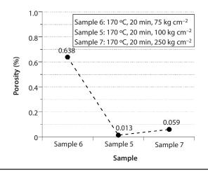
Figure 10 Porosity in banana fiber-reinforced composites processed under various pressures.
