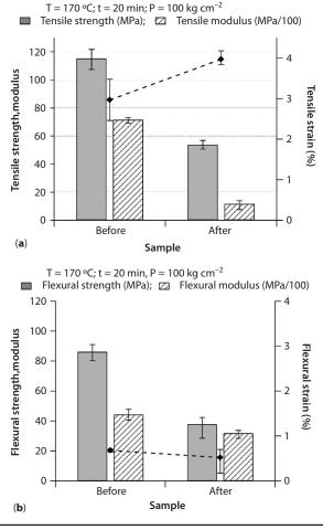
**Figure 14** (a) Tensile and (b) flexural properties of banana fiber-reinforced composites prepared at T = 170 °C,  $P = 100 \text{ kg cm}^{-2}$  in 20 min before and after water absorption.
