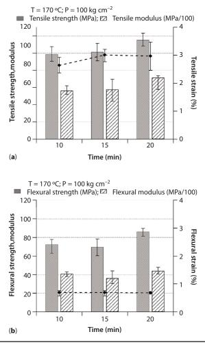
**Figure 5** Effects of processing time on (**a**) tensile and (**b**) flexural properties of banana fiber-reinforced composites.
