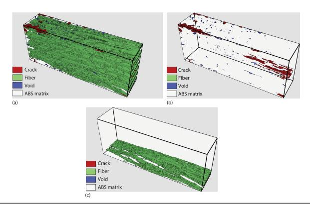
**Figure 9** A banana fiber-reinforced composite processed at 170 °C in 20 min and under 125 kg cm<sup>-2</sup>: (**a**) Three-dimensional whole structures, (**b**) void and crack distribution, and (**c**) 3D structure of one layer.
