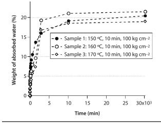
Figure 4 Water absorption of banana fiber-reinforced composites processed at various temperatures.
