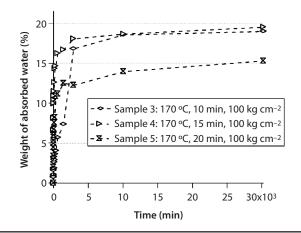
Figure 7 Water absorption of banana fiber-reinforced composites processed in various times.
