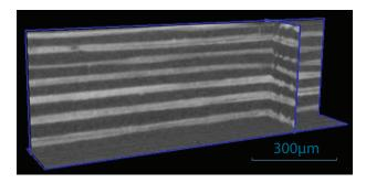
**Figure 12** 3D model reconstruction of a banana fiberreinforced composite prepared at T = 170 °C, P =  $100 \text{ kg cm}^{-2}$  in 20 min.
