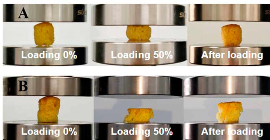
Figure 5: Compression test images of (A) DGDHAA/ESO-BAPA1.0 and (B) DGDHAA/ESO-BAPA1.2.
