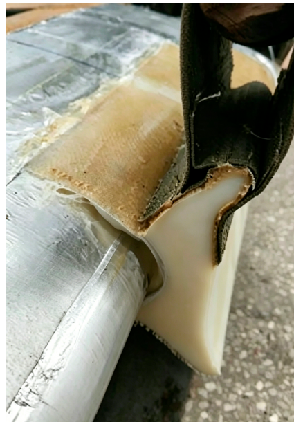
Figure 18: The failure mode of simulated ice.
