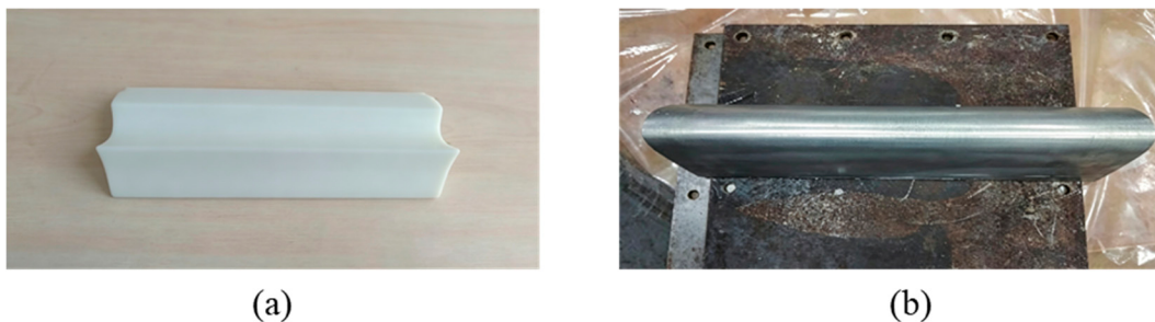
Figure 17: Test components: (a) 3D-printed ice core; (b) aluminum fixture.
