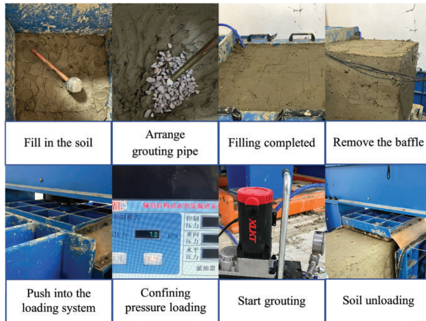
Figure 4: Schematic representation of grouting test procedure
