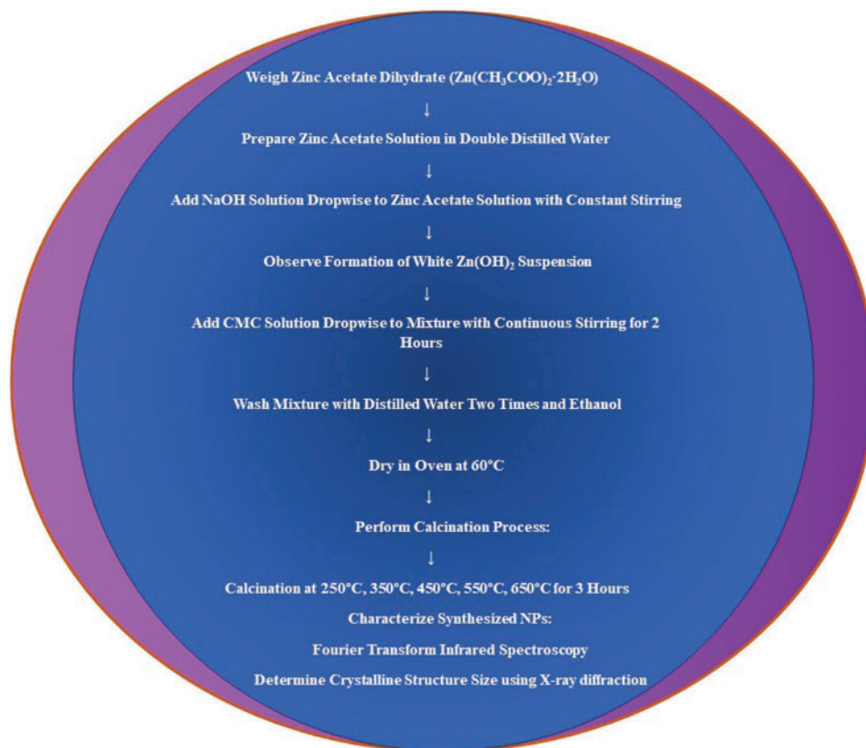
Figure 2: Flow chart showing the synthesis of CMC-wrapped ZnONPs
