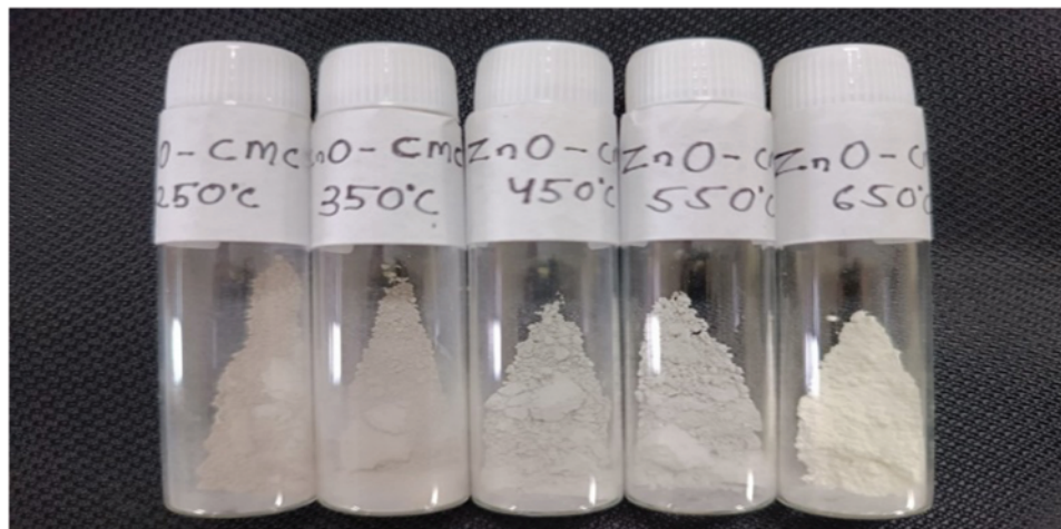
Figure 3: Synthesized ZnONPs @CMC samples at various calcination temperatures
