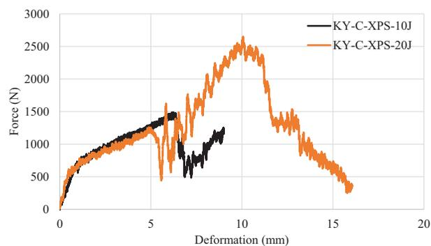
**Figure 8:** KY-C-XPS force-deformation graph under 10 and 20 J impact energy
