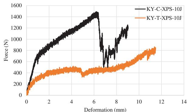
**Figure 5:** Force-deformation graph of single and double layer samples with XPS core material as a result of 10 J impact energy
