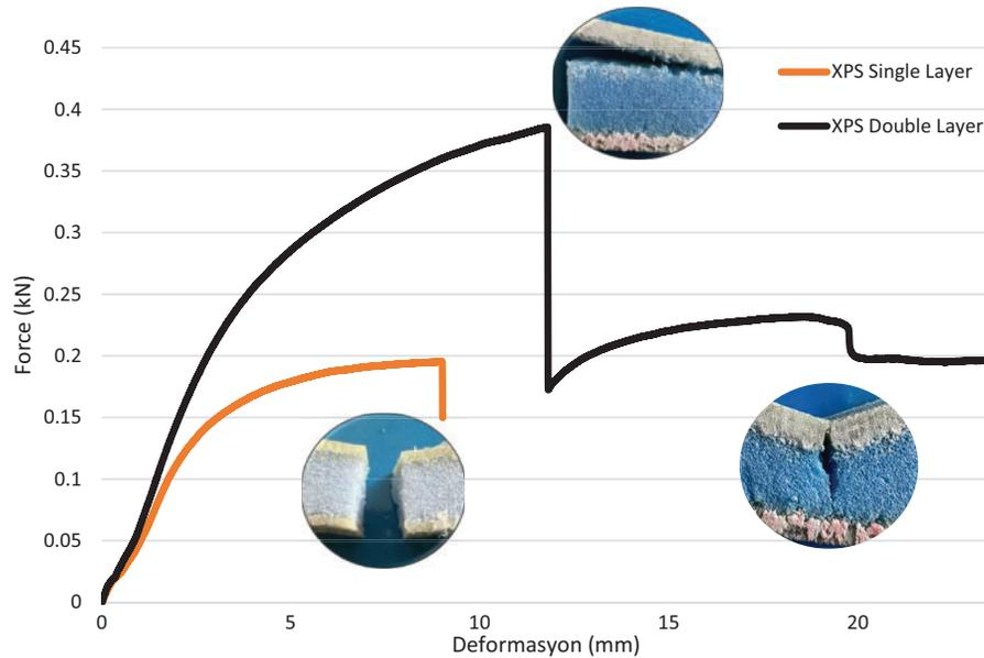
**Figure 12:** XPS force-deformation graph
