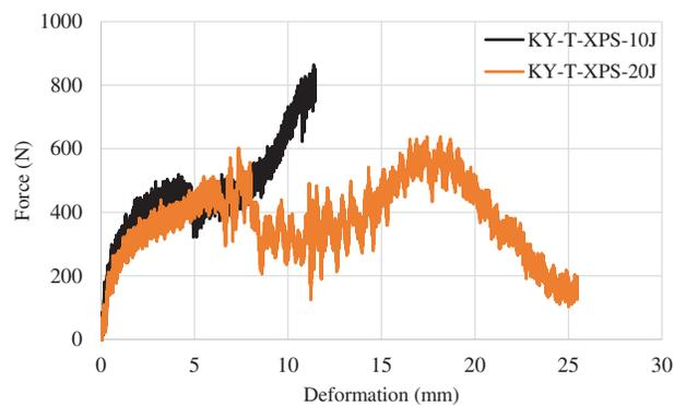
**Figure 7:** KY-T-XPS force-deformation graph under 10 and 20 J impact energy
