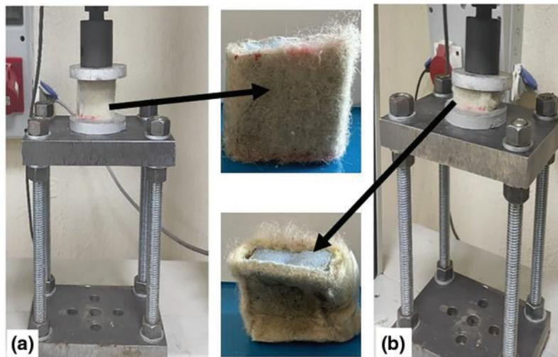
**Figure 9:** XPS sheep wool (a) Before the compression test (b) After the compression test
