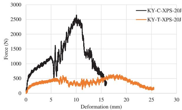
**Figure 6:** Force-deformation graph of single and double layer samples with XPS core material as a result of 20 J impact energy
