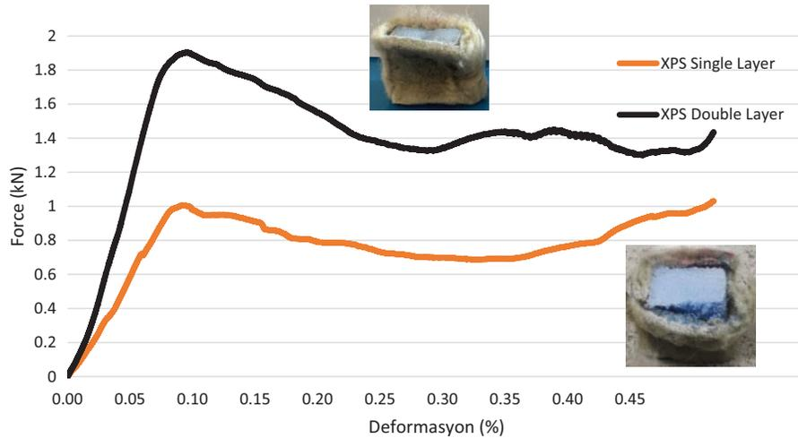
**Figure 10:** XPS single and double layer compression test force-deformation graph
