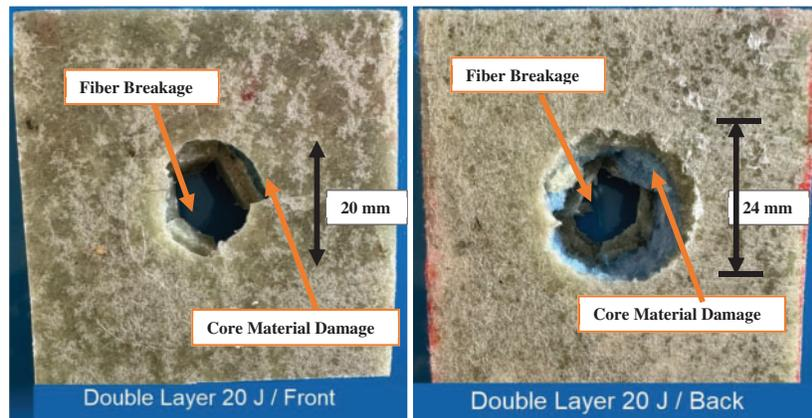
**Figure 4:** XPS sample damage images as a result of the impact test
