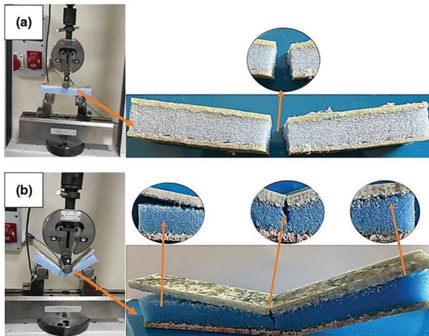
**Figure 11:** Compression test of XPS sheep wool sample (a) Single layer sample (b) Double layer sample
