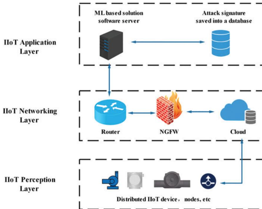
**Figure 1:** Solution based on IDS network architecture in IIoT environment
