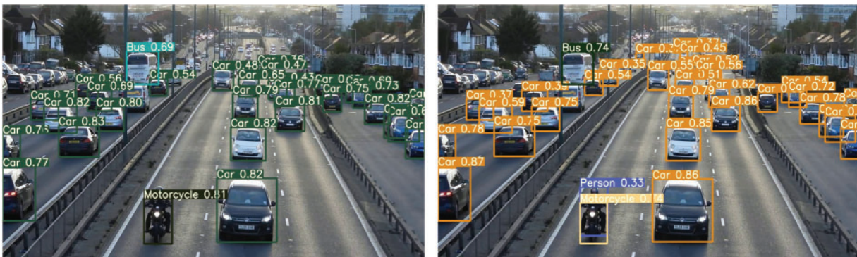
Figure 10: The detection result for YOLOv7 for original dataset and Exp_5 models at day-light time
