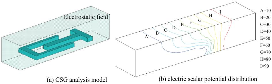
Figure 3: Electrostatic analysis of a comb drive case (one pair of fingers, unit: Volt)
