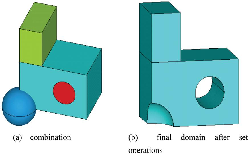
Figure 1: Regular three-dimensional analysis domain by set operation
