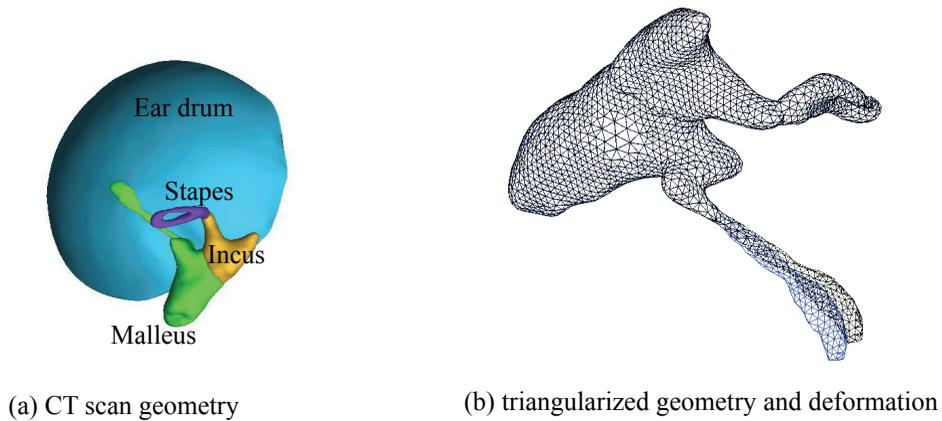
Figure 4: Structural analysis of ossicles of middle ear
