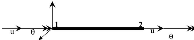
(b) One dimensional beam element showing axial degrees of freedom (two) at each nodes
