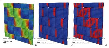
FE modeling of tension (horizontal) of woven carbon-epoxy composite: (a) transverse stress in yarns, applied strain 0.29%; (b,c) damaged elements (transverse damage), applied strain 0.29% and 0.52%. Damaged elements: red.
