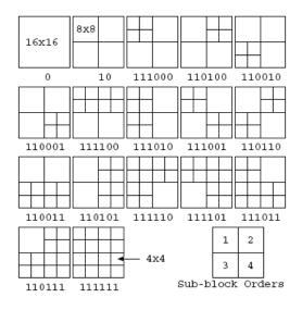
Figure 2: All possible 16 x 16 block partitioning modes
