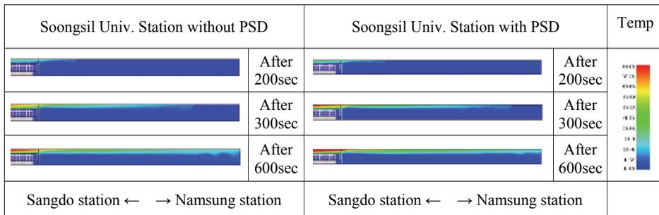
Figure 7: Transient temperature distribution in the Namsung-direction train-way of the Soongsil Univ Station after fire (Y=14.04m)
