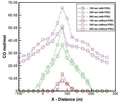
Figure 8: Transient CO concentration along trainway (Z=6.18m)
