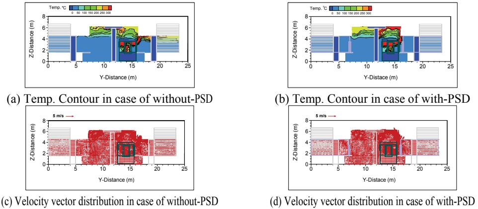
Figure 10: The Temp. Contour and velocity vector distribution of the Platform Vertical Section (X: 85m, 600 sec)
