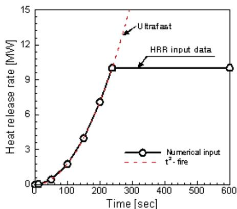
Figure 5: Ultra fast mode for HRR input
