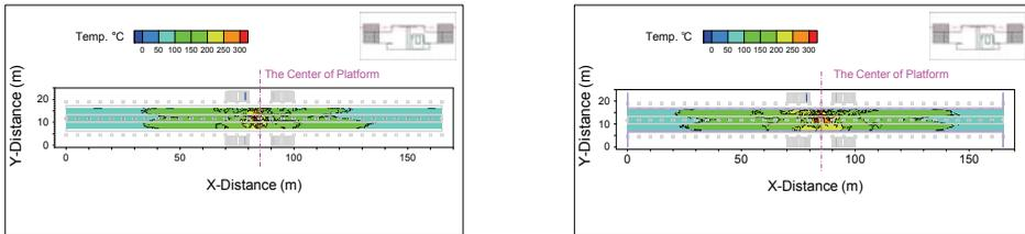
(a) Temp. contour in case of without-PSD
