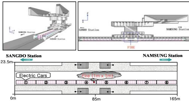
Figure 4: Model and fire location for Soongsil Univ. station
