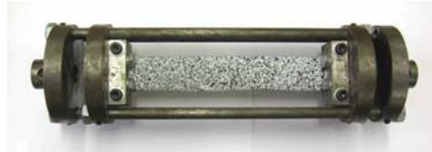
Figure 1: Loading cage for buckling specimen
