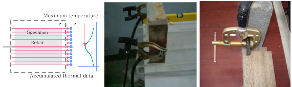
Figure 3: Accumulated thermal data Figure 4: Plier type earth clamp Figure 5: Vise type earth clamp
