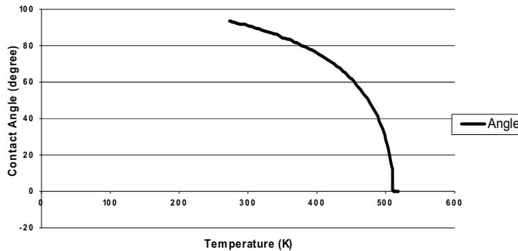
Figure 2: A plot of contact angle versus temperature for the water-air-graphite interface.
