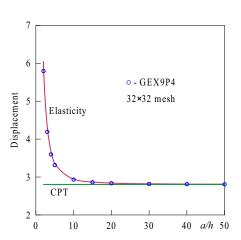
Figure 2: Transverse displacement at center point  $100Eh^3u_{30}^M/p_0a^4$  of rectangular homogeneous plate.
