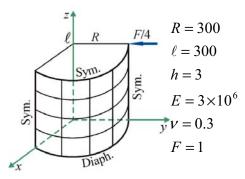
Figure 4: Pinched cylindrical shell with rigid diaphragms
