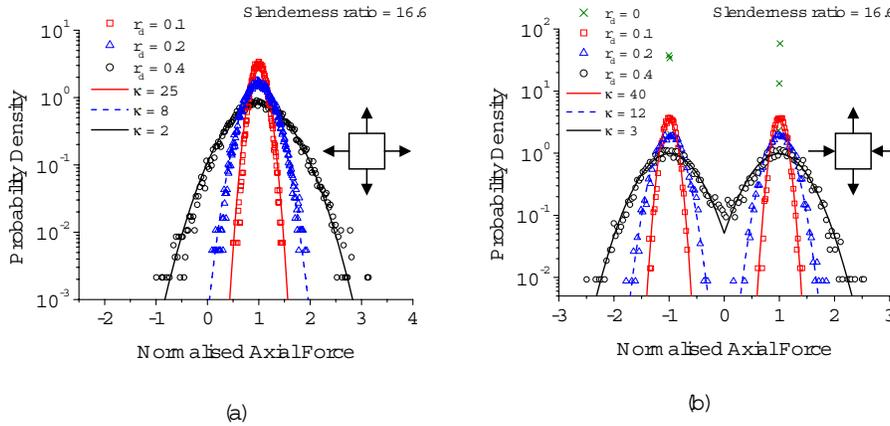
Figure 3: Axial force distributions in 2-D grids calculated using finite element simulation under (a) hydrostatic loading and (b) biaxial pure shear loading.
