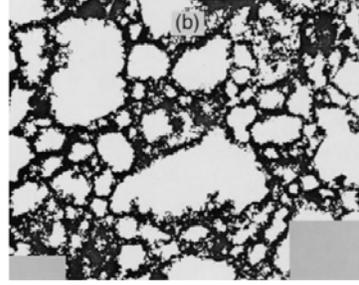
Figure 6: Predicted steady-state dislocation density distribution [15]. Figure 7: Experimental fractal pattern of dislocations [16].
