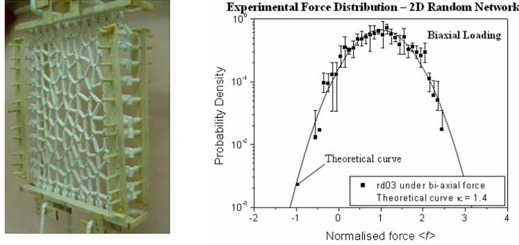
Figure 1: Experimental measurement of axial force distribution in 2-D elastic networks. The left panel shows the experimental setup [11]. The network is made of silicone and the axial forces in the members inside were measured from the displacements of the nodes upon load application.
