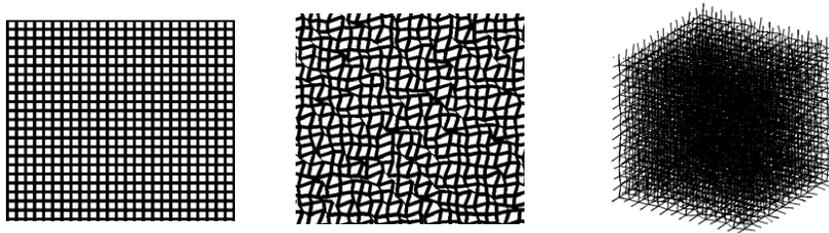
Figure 2: 2-D and 3-D grids used in finite element simulation. First grid has  $r_d = 0$ . The last two grids have  $r_d = 0.4$ .
