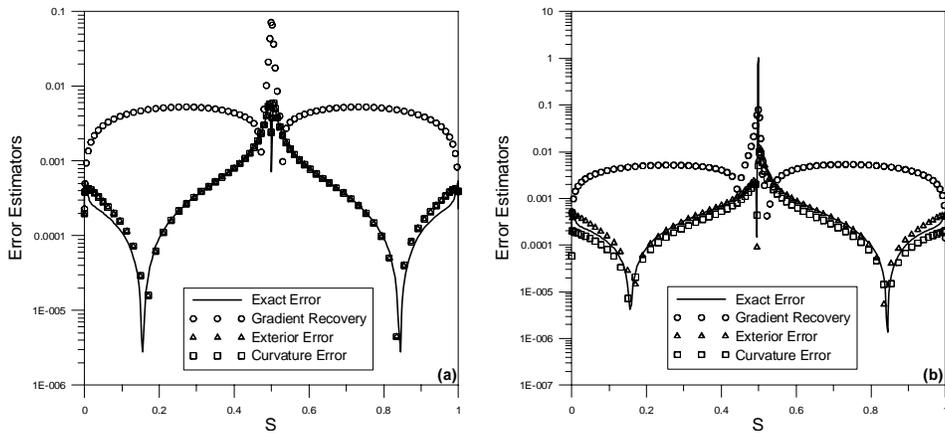
Figure 1: Joukowski airfoil without camber, for  $n = 300$  linear panels, and for two different attack angles: (a)  $\alpha = 0^\circ$  and (b)  $\alpha = 3^\circ$ .
