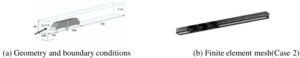
Figure 7: Flow around a railway vehicle in a tunnel
