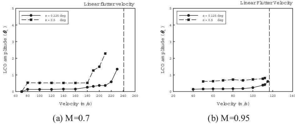
Figure 3: Comparisons of the LCO amplitude between  $s=0.125^\circ$  and  $0.5^\circ$ .
