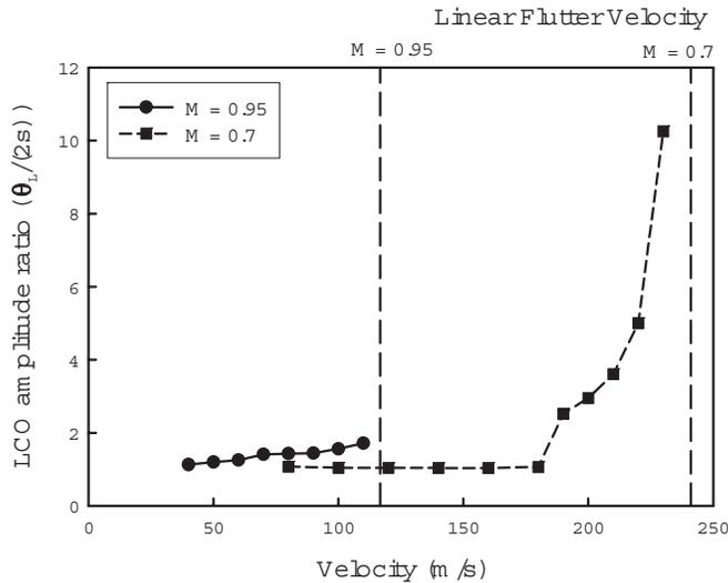
Figure 1: Velocity vs the LCO amplitude ratio.
