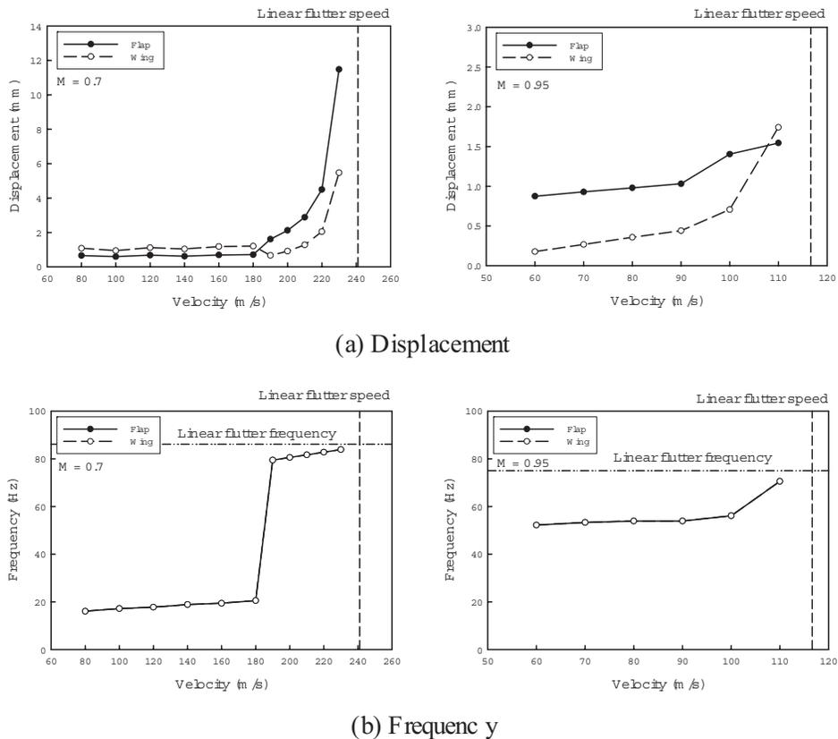
Figure 2: Displacement and frequency of the flap and wing.
