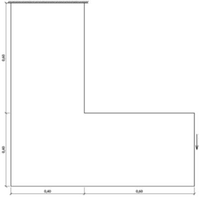
Figure 1: L-shape beam (units in meters).
