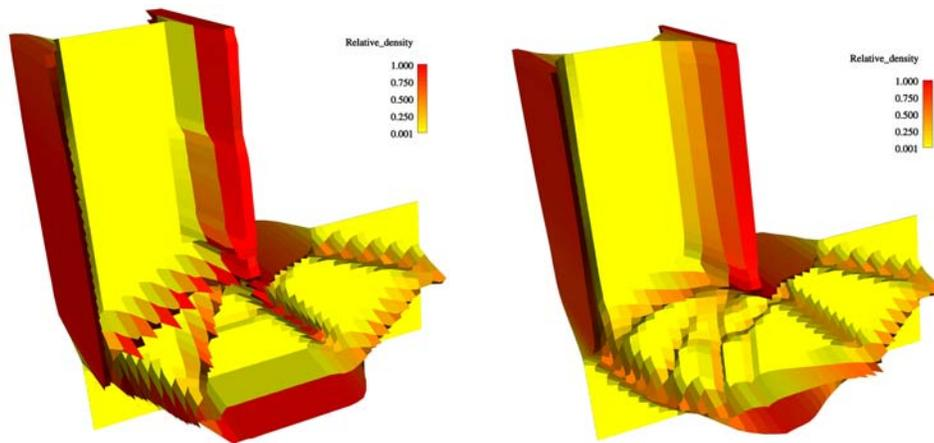
Figure 2: Local approach with  $q=1$  ( $F=18.2\% F_0$ ) (left) and global approach  $\mu = 20$ , ( $F=17.6\% F_0$ ) (right),  $\varepsilon = 0.01$  and  $p = 4$ , (Thickness multiplied by a factor of 0.5) and Bendsøe [8].
