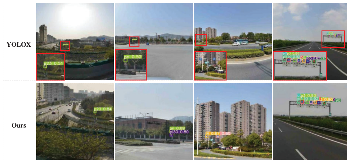
Figure 12: Before the improvement, the base network YOLOv5 and YOLOX had the phenomenon of missing detection for small objects
