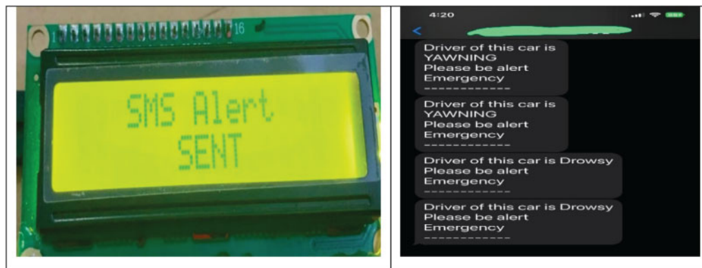
Figure 13: Alert message sent and shown on the mobile phone
