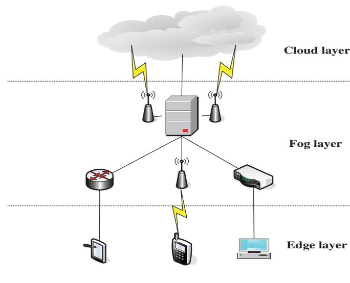
**Figure 2:** Fog computing architecture
