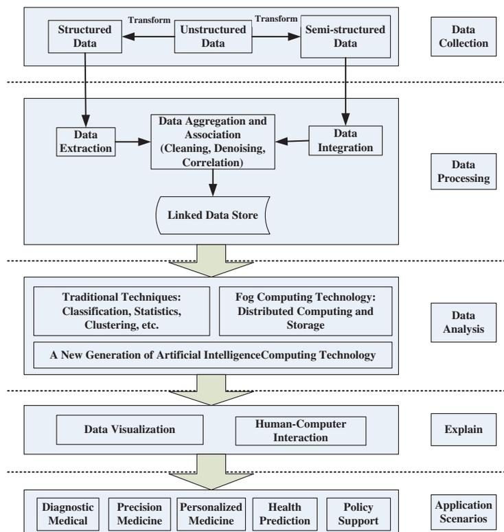
**Figure 1:** Medical big data processing architecture
