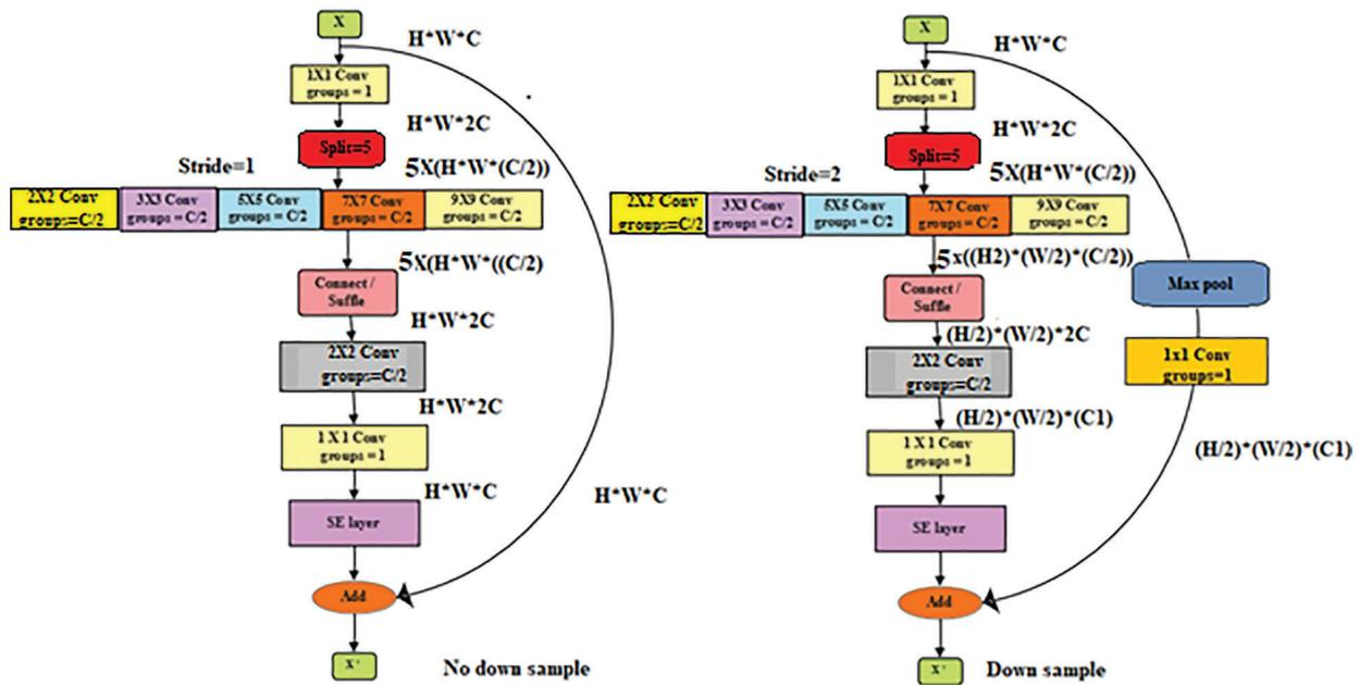
**Figure 5:** Multi-scale residual module
