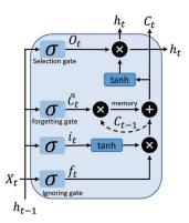
Figure 2: The internal structure of LSTM cell
