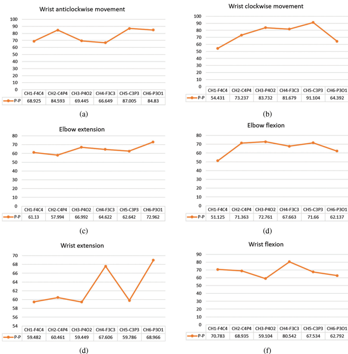
Figure 7: Peak-to-peak values of (a) wrist anticlockwise movement (b) wrist clockwise movement (c) elbow extension (d) elbow flexion (e) wrist extension (f) wrist flexion
