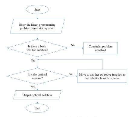
Figure 1: Proposed algorithm flowchart
