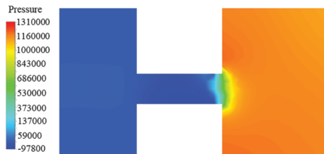
Figure 12: Pressure contour of the jet impingement-negative pressure ammonia removal reactor
