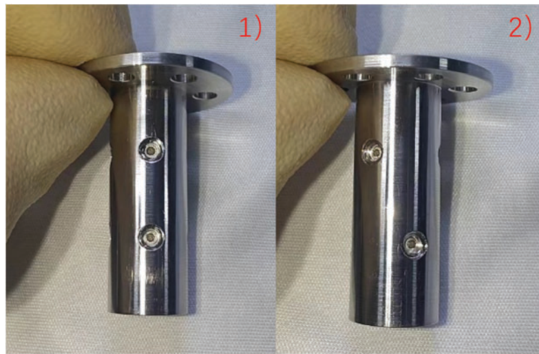
Figure 13: Physical picture of two kinds of piston test samples. (1) 2 \times 4 aerostatic hole layout; (2) 2 \times 3 aerostatic hole layout
