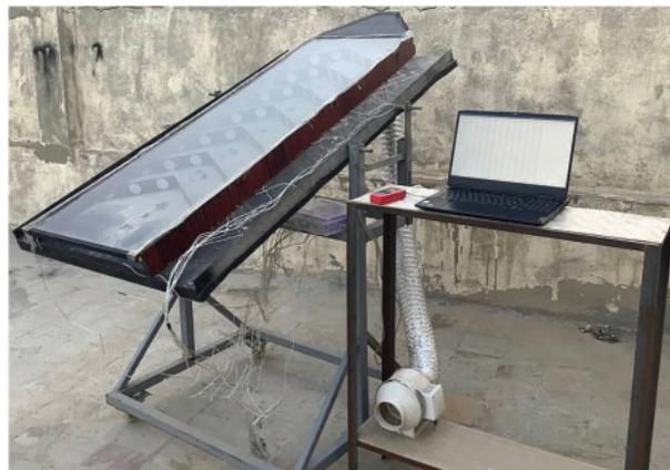
**Figure 2:** Physical construction of solar air heater system
