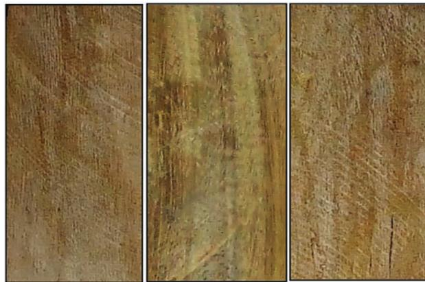
**Figure 8:** External shape of samples heated under IMWH (Left: at 300 watts; Center at 500 watts; Right at 1000 watts)
