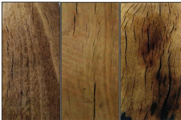
**Figure 7:** External shape of wood samples heated under CMWH scenario (Left at 300 watts; Center at 500 watts; Right at 1000 watts)
